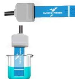
(9) Immerse the strip sampling port end into the test sample until the white line. If you have a CS200 mixer, you can attach the Extended Connection Cable to the bracket.
